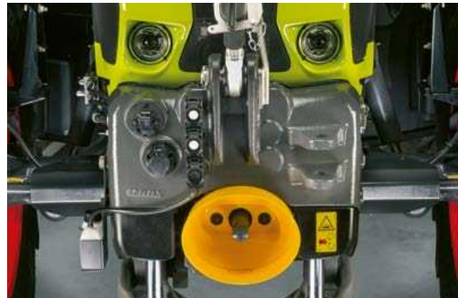
The front linkage has connections for one spool valve and one free-flow return line.
