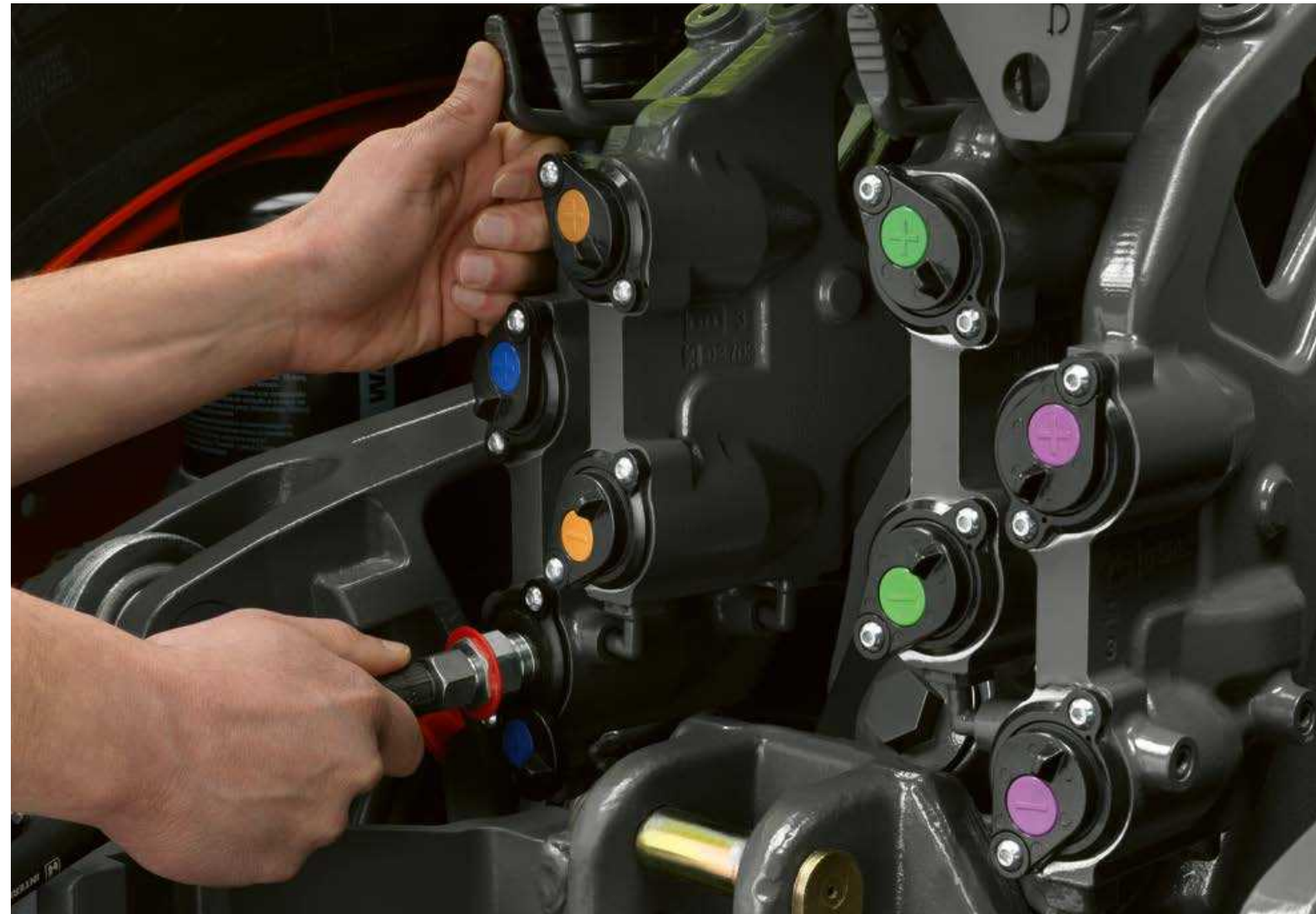
The front linkage has connections for one spool valve and one free-flow return line.
