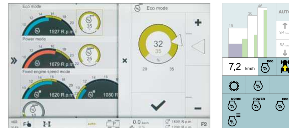
Engine droop setting for "Eco" and "Power", and the engine speed memory.
