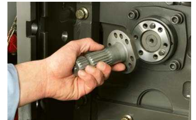
The PTO stub can be changed easily.
