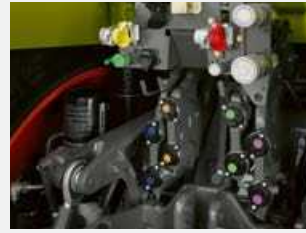
Air brakes with air drier.
