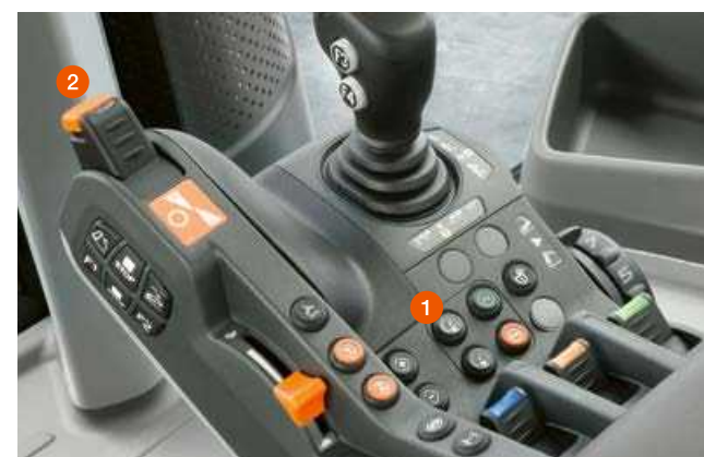
CIS+ operation 1 Change range 2 Activate cruise control
