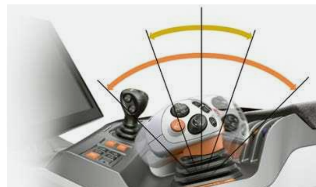
Shifting operation Powershift speeds + / -
