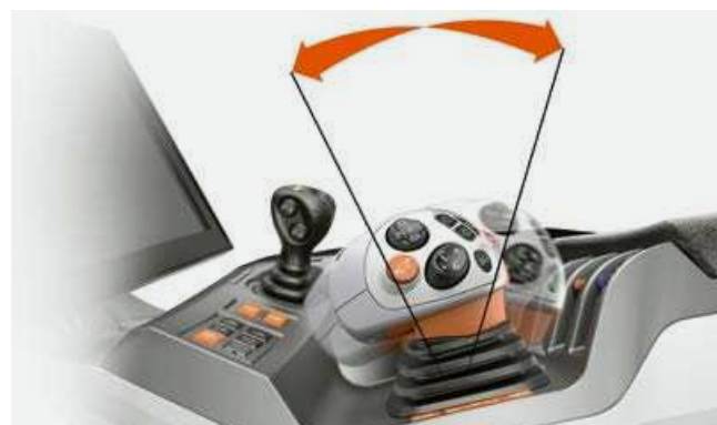
Progressive operation with CMATIC continuously variable transmission technology.
