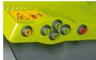
External controls for the rear linkage, PTO and one freely selectable spool valve (CEBIS only).
