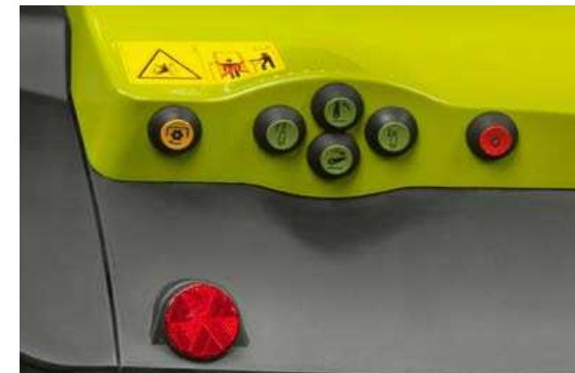
External controls for rear PTO.
